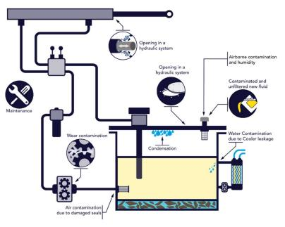
Also, water shouldn't be underestimated as it is a serious contamination type that leads to issues like fluid oxidation, internal surfaces corrosion, additive depletion and many more fluid failures. These failure modes will cause acceleration of the degradation process of the oil.
