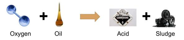
Thermal degradation happens because of the chemical change in base oil molecules at high temperature. Thermal failure occurs whenever the oil touches a machine at elevated temperatures.
