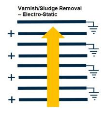
**Balanced Charge Agglomeration** (BCA) is another way where the separators place a charge on the oil to cause sludge and fine particles to agglomerate so they can be filtered out of the oil. Very effective for removing semi-soluble soft particle and preventing deposits. Affected by moisture contamination.
