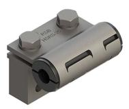
6. Sensor clamps - Fixing clamp for proximity switch according to EN 50025 and 50037. Metal parts of the standard program of series A according to DIN 3105 must be used. The sensors can be adjusted axially and laterally when mounted on mounting rails.
